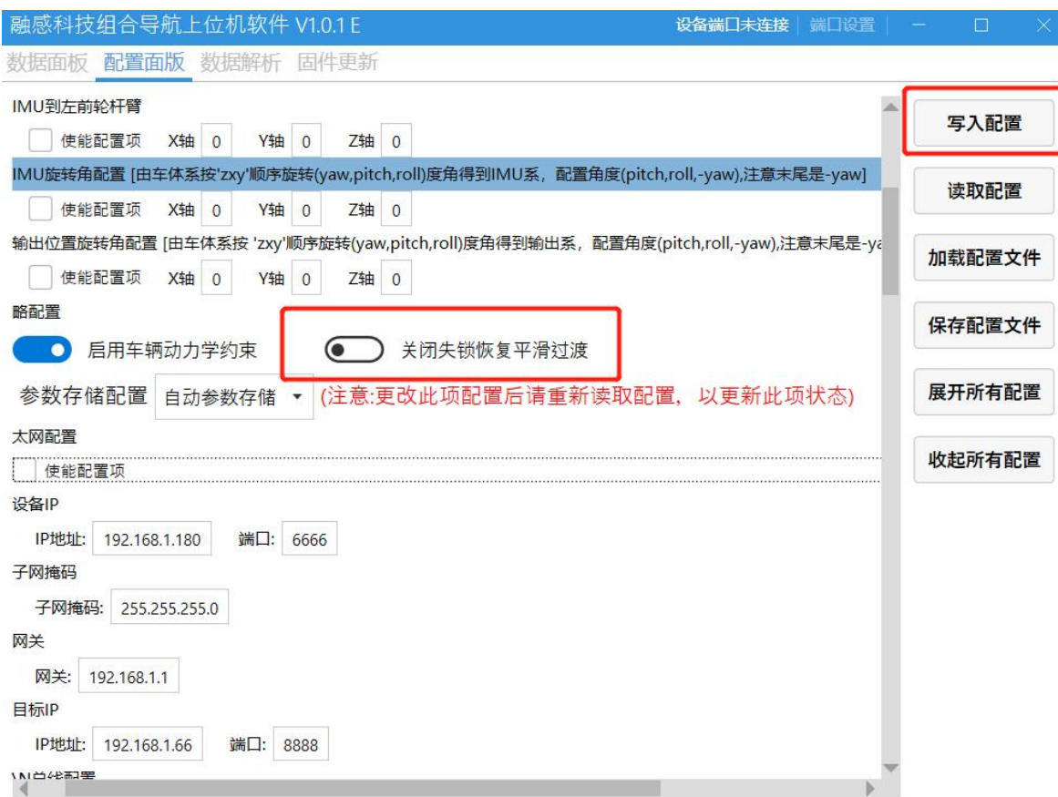
Figure 12 Lock-out recovery smooth transition configuration diagram
