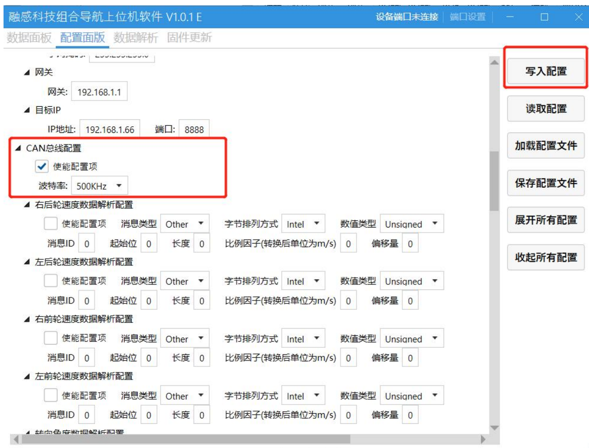
Figure 14 CAN port parameter configuration diagram
