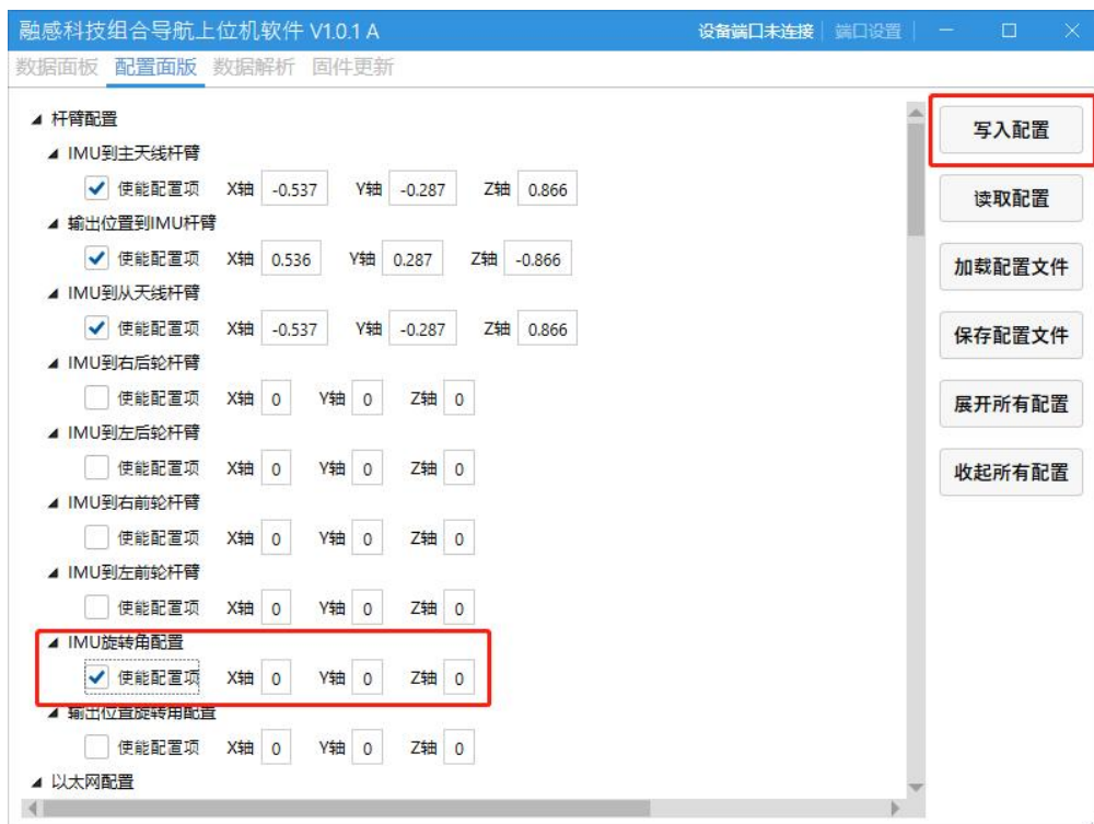
Figure 9 Rotation angle parameter configuration diagram
