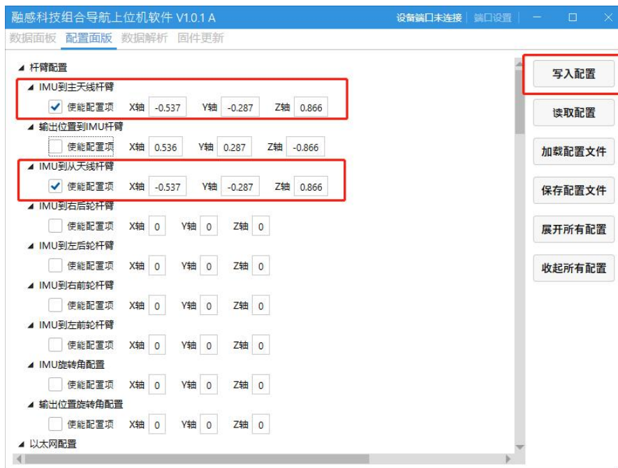
Figure 5 Parameter configuration diagram of the antenna rod and arm value
