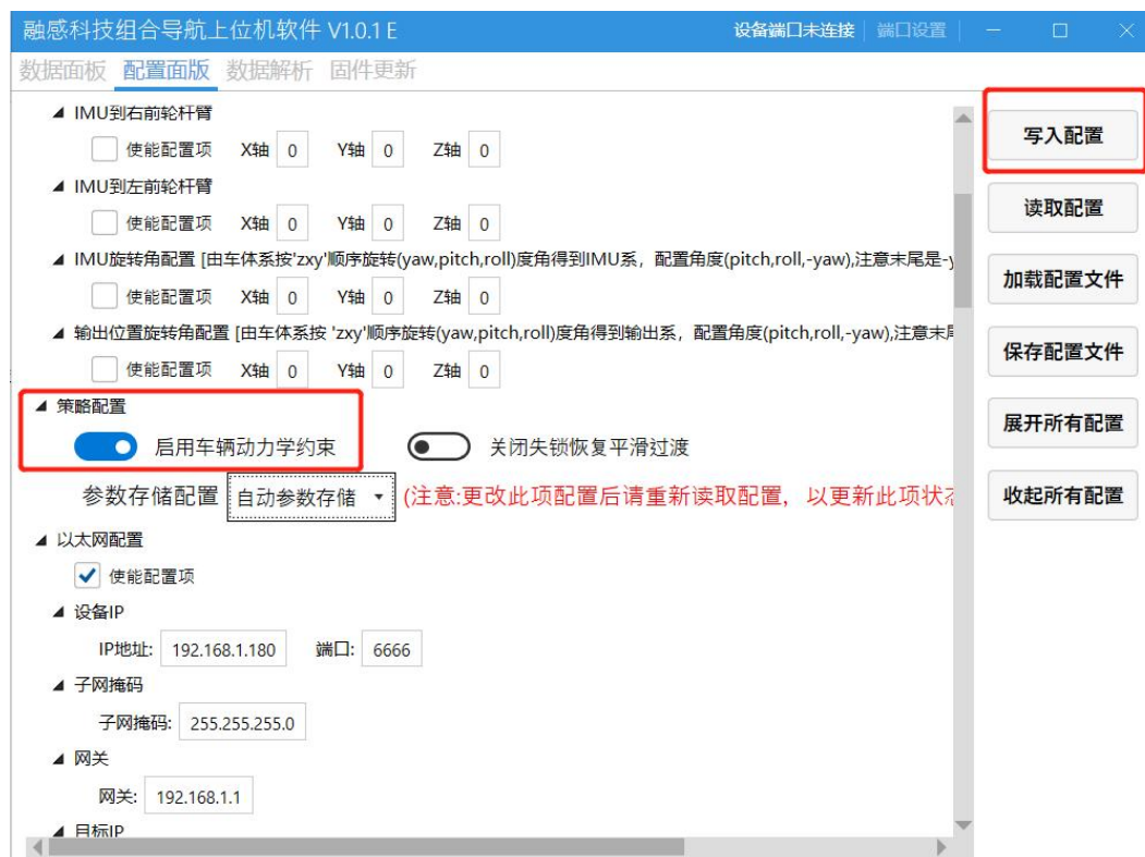
Figure 11 Vehicle dynamics constraint configuration diagram
